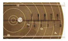
for ease of reading. The gauge is inserted in the target in the same way as the decimal gauge. However in this case the number of tenths to be added is determined by which of the numbered, engraved lines aligns with a line on the target. If no line aligns accurately, then the value is that of the nearest line *just inside* a scoring ring on the target, e.g. 10.1 in the illustration above.
