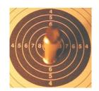
The NSRA 6 yard air rifle and ISSF 10 metre air rifle gauge (the same gauge is used for both targets) and the NSRA 6 yard air pistol gauge score by reference to the second ring out. Thus if the outside edge of the gauge falls within the 7-ring and outside the 8-ring, the shot value is 9 points.
